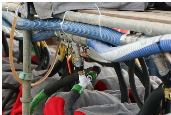
Tee/valve assembly with CBF adaptor and CAMRA pipework
