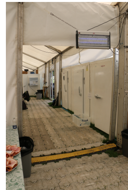
Ramp recessed with closely surrounding floor, minimizing trip-hazard; bug-zapper at a good height (2 m) on entry to food area
